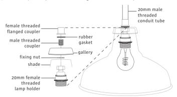
**CAUTION:** Use suitable thread-locking fluid to prevent rotation and loosening of threaded parts between lamp holder and conduit
