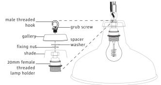
**CAUTION:** Use suitable thread-locking fluid to prevent rotation and loosening of threaded parts between lamp holder and hook
