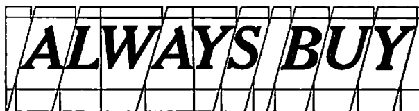
Fig. 95. Intertype Display Italic Matrices are of a special angular-cut design which makes it possible to fit the characters closely together. When the matrices are assembled, the angular cuts dovetail and the matrix characters are located properly with respect to each other. The precise spacing and proportion of characters demanded for advertising composition and other classes of display work are thereby obtained. Special opening and closing quads and hair spaces are provided for use with display italic matrices.
